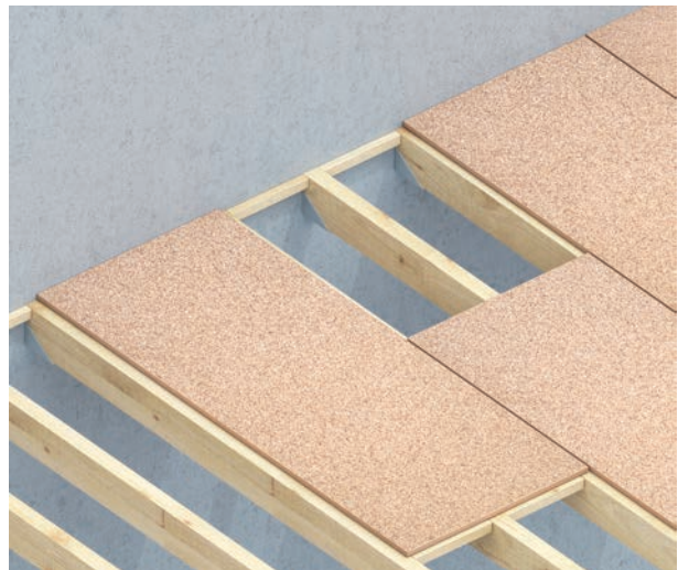
FIG. 2: Modulation for floor slab
