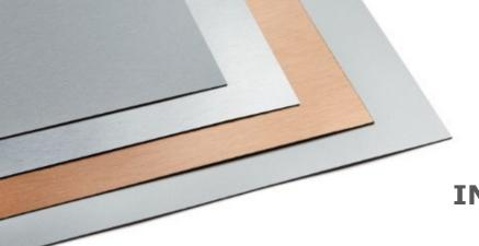
Innovus Metallic laminates are high-pressure decorative laminates according to EN 438 with metal surface. Aluminium surfaces are coated with an epoxy lacquer and copper surface coated with a polyurethane lacquer. Innovus Metallic are intended for use in vertical and light duty interior applications.
